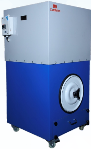
NORMAL/PORTABLE RANGE OF MODEL CAPACITY FROM 300 CFM TO 1200 CFM SUCTION PRESSURE: FROM 80 MM WG TO 400MM WG
